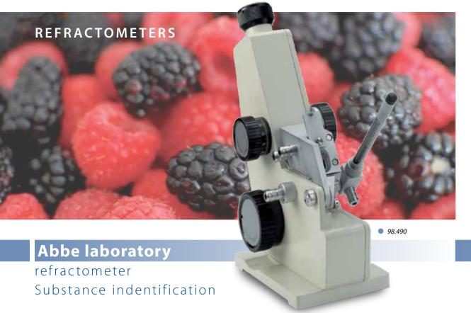
The Abbe laboratory refractometer is a bench-top instrument for high-precision measurements of an index of refraction. The Abbe refractometer is also suitable for determination of the refractive index of solid samples, such as glass, plastics, and polymer films. The instrument is equipped with a built-in thermometer and water connection to control fluid temperatures. Also equipped with a Brix and a refraction index scale and supplied with a test plate
